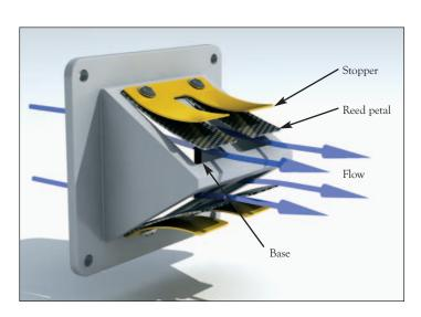
A diagram of a reed valve, showing the flexible reed petal, base, and stopper
