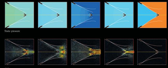
Velocity vectors The flow field in a reed valve at various times for an engine running at 4770 RPM
