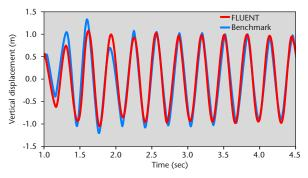
The vertical displacement of the beam free end predicted by the FSI model is compared to reference data (1, 2)
