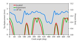
Tip displacement of an engine reed valve predicted by the FSI model and measured experimentally (4); the measured pressure differential is also shown
